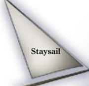
**Fore-and-aft sails** are mounted along the length of the vessel. Acting like the airfoil of an airplane wing, they shape the wind into areas of high and low pressure that pull the ship forward. They are efficient at catching wind from all directions and are critical in steering the ship.
