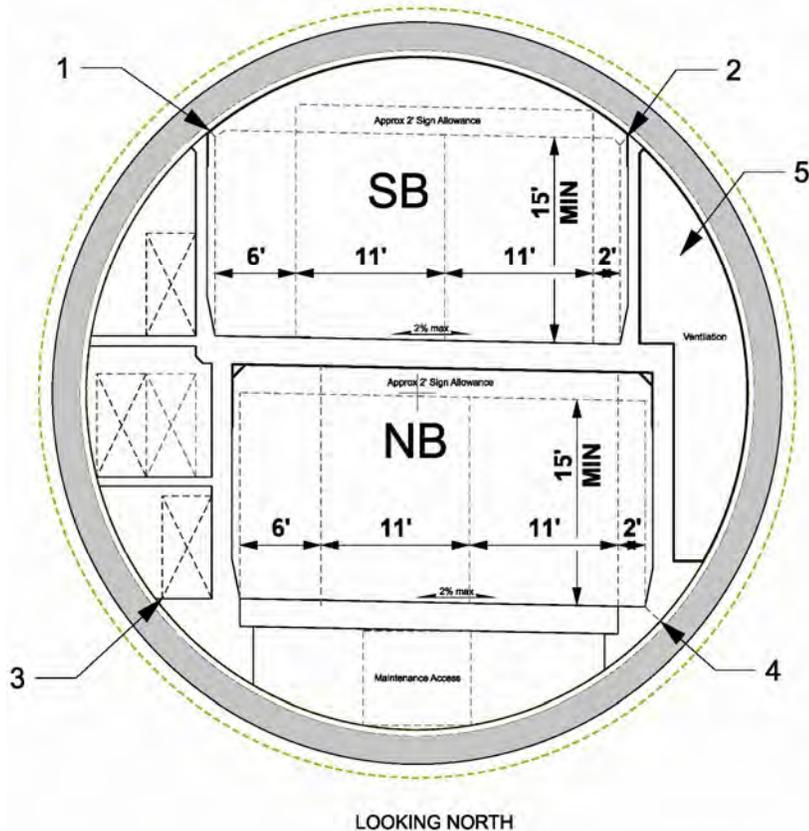
Figure 3. General Tunnel Cross-section Identifying Critical Points
