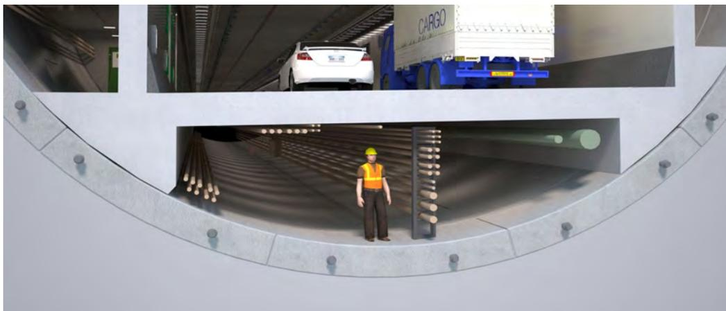
**Figure 5. Typical Cross-section - Lower Maintenance Access**
