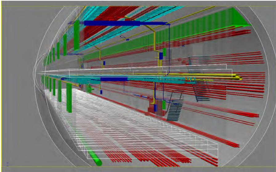
**Figure 7. Computer Rendering of 3D Space Proofing of Tunnel Utilities**
