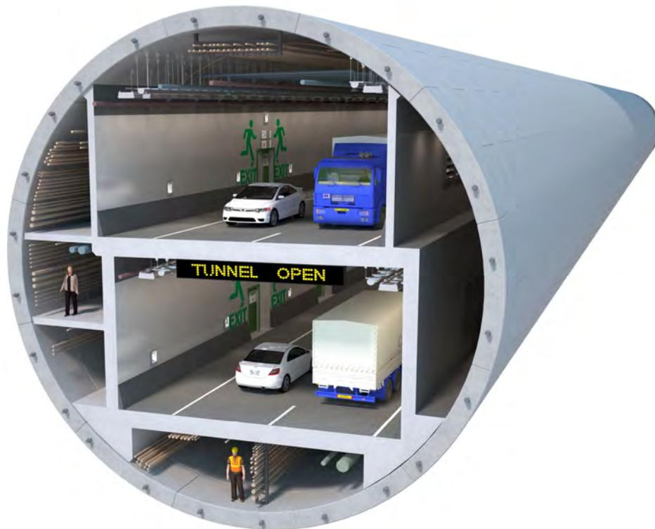
**Figure 2. Proposed Bored Tunnel Cross-Section**
